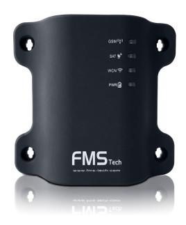
The Track 360 is a powerful device with Global Navigation Satellite System (GNSS) which supports both GPS and GLONASS in order to provide accurate data and faster connecting. Through these systems the user can have notifications sent quickly to their computer or mobile device. This device is an economical choice since the number of inputs is limited compared to other options, however this
