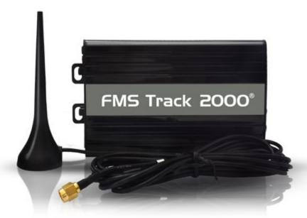
The FMS Track 2000 is a powerful On-board Computer that combines vehicle routes information with vehicle sensors status and telematics ie. Speedo cable, engine RPM, etc., and location based information suitable for OFFLINE applications. Fleet manager can obtain vehicle and trip information and alerts OFFLINE on
