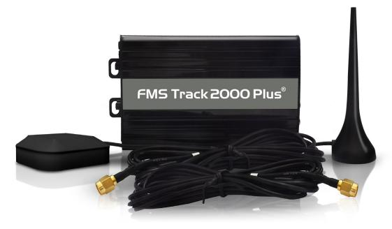
The FMS Track 2K+ Device has Global Navigation Satellite System (GNSS) which supports both GPS and GLONASS in order to provide accurate data and faster connecting. Through these systems the user can have notifications sent quickly to their computer or mobile device. Multiple inputs can connect to various sensors in the vehicle to collect a wide range of telematics and statistics, while the onboard CAN BUS allows the user to have easy access to any detail of the vehicle.
