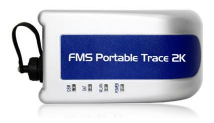
The FMS Portable Trace 2K is the modified and simpler version of the existing FMS Trace 2k product however the FMS Portable Trace 2K features GPS and GPRS and 4 digital inputs only. The FMS Portable Trace 2K DOES NOT come with RFID, Driver Access Card, Zigbee wireless, Buzzer, or Ignition Relay.
